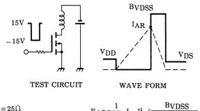
$$\begin{array}{ll} R_{\text{G}}\!=\!25\Omega \\ V_{\text{DD}}\!=\!-50\text{V}, \; L\!=\!747\mu\text{H} \end{array} \qquad E_{\text{AS}}\!=\!\frac{1}{2}\cdot\text{L}\cdot\text{I}^2\cdot(\frac{\text{BVDSS}}{\text{BVDSS}-\text{V}_{\text{DD}}})$$
